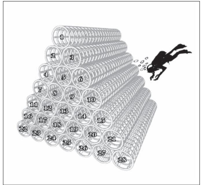
Fig. 3. Schematic drawing of the 'cross-hatched' benthic artificial reef (Drawing: G. Spanier)
