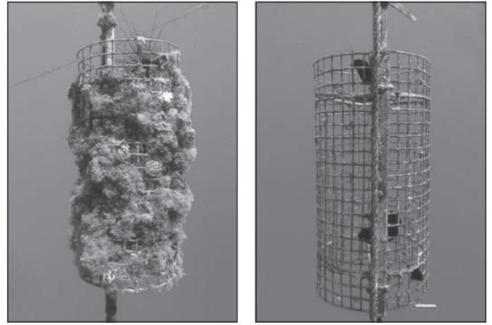
Fig. 6. Bio-filter from site FF (left) compared with one from site R (right), February 2002 (Photo: S. Breitstein)
